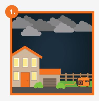
NEVER OPERATE A PORTABLE GENERATOR INDOORS, IN HOMES, GARAGES, BASEMENTS, CRAWL SPACES OR OTHER ENCLOSED OR PARTIALLY ENCLOSED AREAS, EVEN WITH VENTILATION. ALWAYS USE GENERATORS OUTDOORS, MAINTAINING A SAFE DISTANCE AWAY FROM DOORS, WINDOWS AND VENTS.
